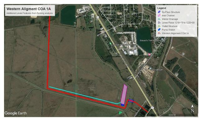
Figure 9-Western Levee Alignment COA 1-A and features
